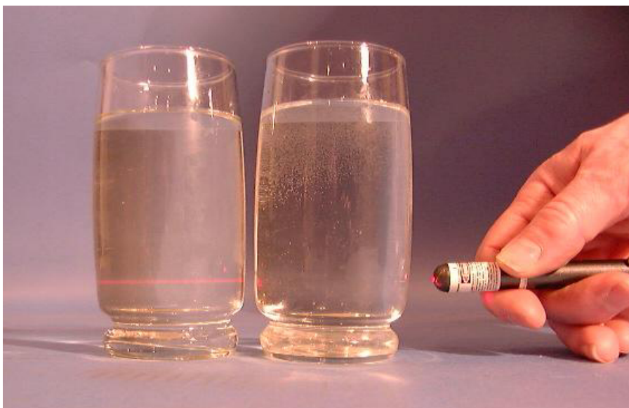
Figure 6.4. Tyndall effect: In the solution (right glass) the light path is invisible, while for the colloid (left glass) the light path is visible 74 .
